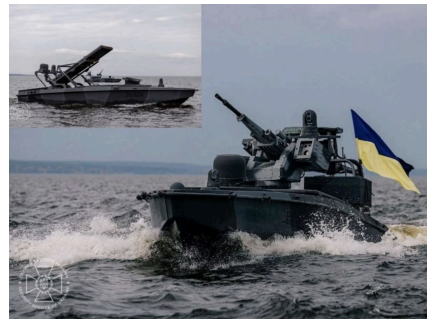
Ukrainian Sea Baby naval drone with a machine-gun mount. Source: SSU
