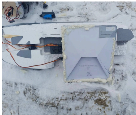
Downed BM-35 UAV With Integrated Starlink. Source: serhii_flash
