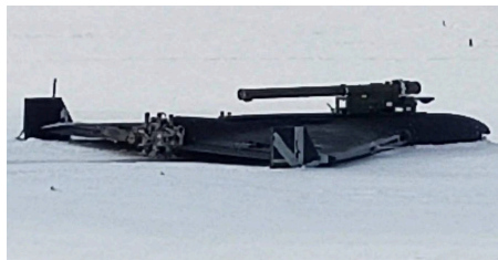
Downed Russian Geran-2 UAV With Integrated Verba MANPADS. Source: serhii_flash
